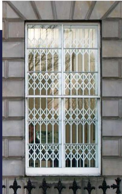
Extendor Vulcan retractable security grilles are certified by the LPCB to LPS 1175 SR2, and are a Secured by Design 'Police Preferred Specification'. As such, these grilles are insurance approved, and have been successfully bomb blast tested in conjunction with glass backed anti-shatter security film. The Vulcan and Eclipse grilles are the only security grilles certified to protect against bolt cutters.
