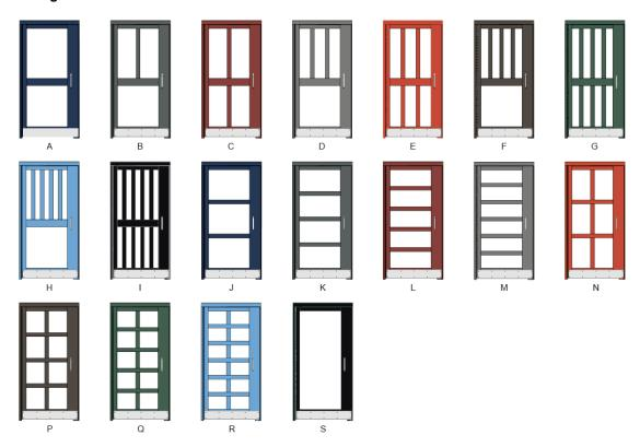
Note: Design configurations are shown with glazed infills, but these can be replaced or used in conjunction with solid infills.
